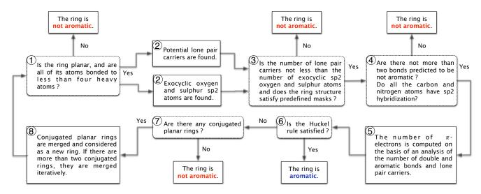
Figure 3: Aromaticity detection workflow.
