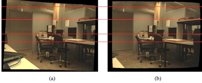
Fig. 30. E-CLUTR corrects distortions as observed on the lines (a) left image (b) right image.
