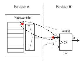
Fig. 10. Example of equivalent fault grouped in a unique partition in order to increase diagnosability
