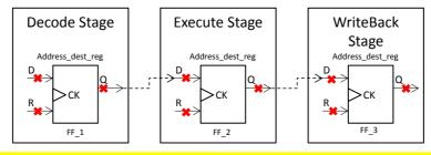
Fig. 6. Example of equivalent faults in different stages of the pipeline; stuck-at faults are highlighted with red x
