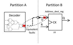
Fig. 9. Example of faults belonging to the same equivalent class traversing two different VLIW partitions
