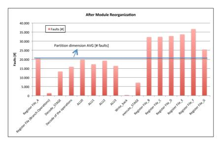
**Fig. 13.** Fault distribution in the different VLIW partitions after the module reorganization phase based on the equivalence classes
