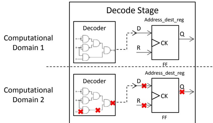
**Fig. 7.** Example of equivalent faults, considering the decoder module of the second computational domain and the decode stage containing all the instruction decode modules; stuck-at faults are highlighted with red x
