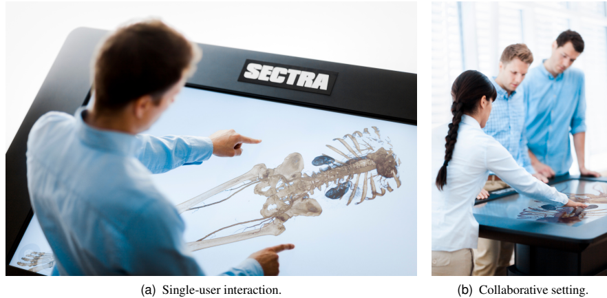
Fig. 16 The virtual surgery table [61], a horizontal interactive surface for the analysis of medical datasets. Image courtesy of and © Sectra, used by permission.
