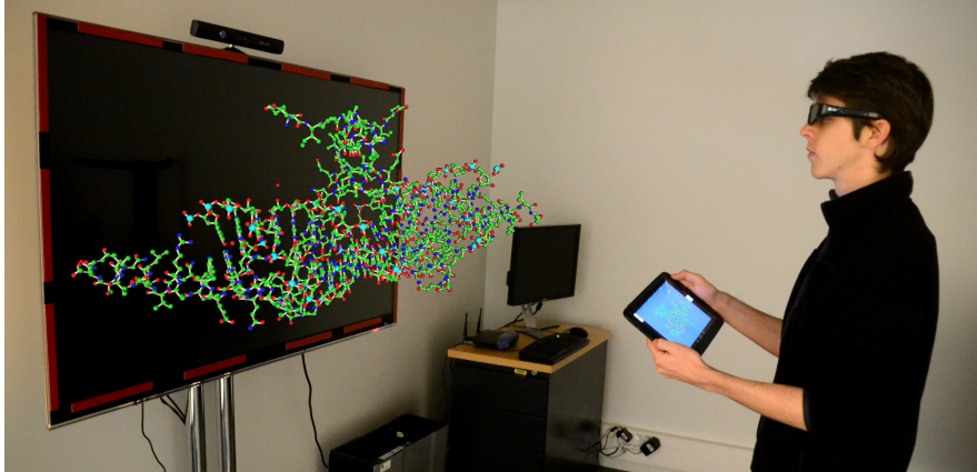
Fig. 3 Stereoscopic data exploration with mobile control. Image from [60], © IEEE, used by permission.
