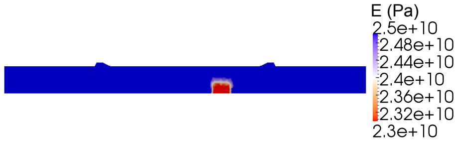
Figure 5: Cartography of Young modulus after Constitutive Relation Error-based model updating process - the damaged area is in red and it corresponds to a 8% damage.
