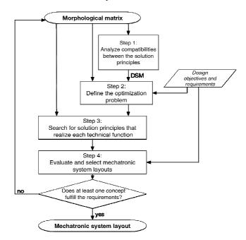
Fig.2. Our optimization-based embodiment design framework
