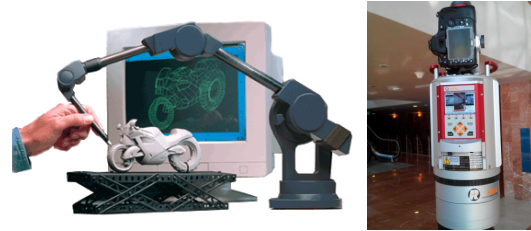
Fig. 1 3D scanning devices. Left: A contact-based MicroScribe device (photo taken from [3]). Right: The Riegl VZ-400 terrestrial laser scanner.
