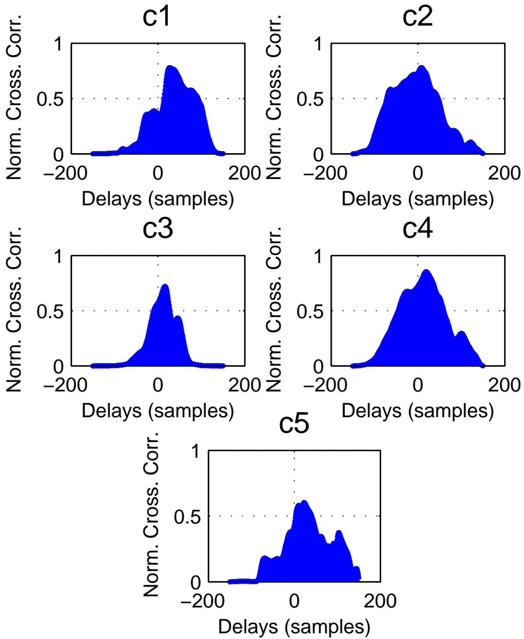
Figure 12: Cross-correlation between the original and optimized  $C(t)$  for the 5-synergy model
