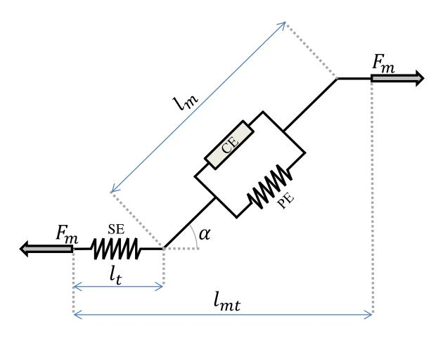
Figure 13: Musculotendon functional model adapted from [17]
