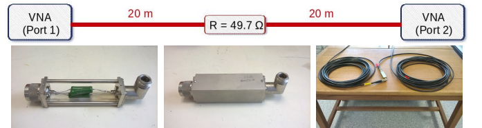
Fig. 3: Case 1: 40m-long cable with a 49.7\Omega resistive fault
