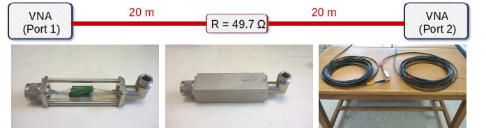
Fig. 3: Case 1: 40m-long cable with a 49.7\Omega resistive fault
