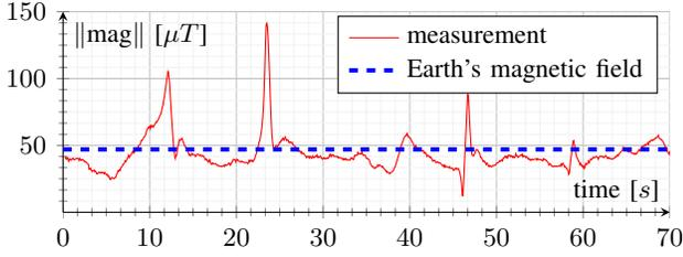
Fig. 3. Magnitude of magnetic field measurements and Earth’s magnetic field in the indoor environment of Inria building in Grenoble.
