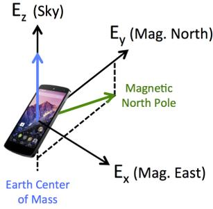
Fig. 1. Reference vectors when the smartphone is static and in the absence of magnetic deviations.
