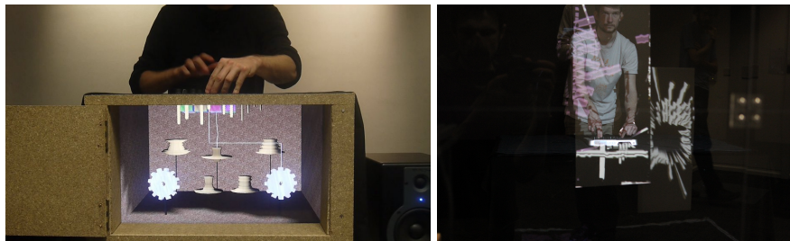
Figure 5: Left: A Digital Musical Instrument is augmented by the Rouages system, revealing its mechanisms. Right: Reflets allows spectators to explore these mechanisms through a large scale semi-transparent mirror.
