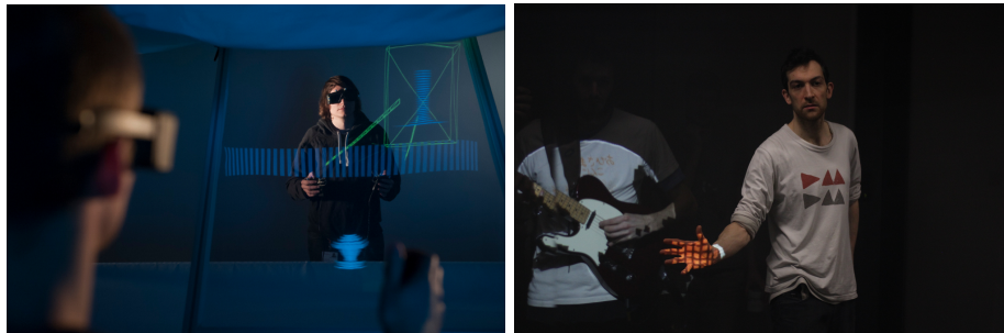
Figure 4: Left: Drile played by two musicians on each side of a semi-transparent 3D screen. The musician on the other side of the screen has selected a reactive widget using virtual rays from his both hands. Right: Two musicians interact through the Reflets system. One musician uses a 3D interface to grab and process the sound of the guitar played by the musician reflected in the mirror.
