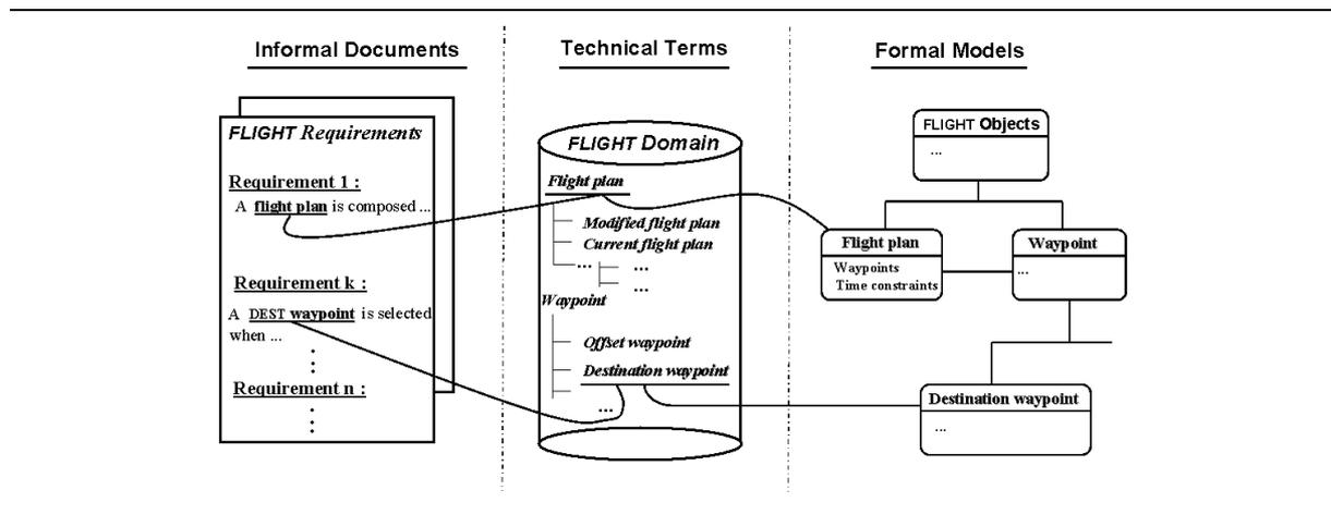
Figure 1. Using terminological items to link textual requirements and object models
