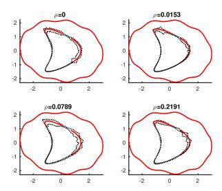
FIG. 9. Reconstruction of two cracks  $\Gamma_0^1 \cup \Gamma_0^2$  in a kite-shaped interface of a two-layered media for four levels of noise  $\rho$ . The solid line at the kite-shaped interface is the exact location of the crack, and the opening between the dotted lines  $\chi_{\tilde{\Gamma}_{\pm}}$  is the predicted location of  $\Gamma_0$ . The outer lighter colored curve is  $\Gamma_1$ .
