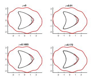
FIG. 8. Reconstruction of a single crack  $\Gamma_0$  in a kite-shaped interface of a two-layered media, for four levels of noise  $\rho$ . The solid line at the kite-shaped interface is the exact location of the crack, and the opening between the dotted lines  $\chi_{\tilde{\Gamma}_{\pm}}$  is the predicted location of  $\Gamma_0$ . The outer lighter colored curve is  $\Gamma_1$ .
