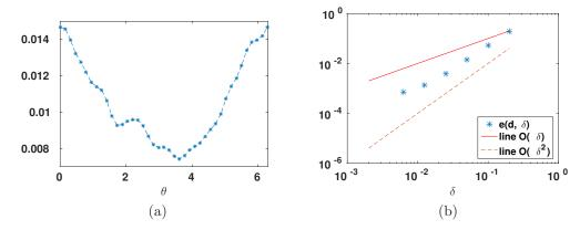
Fig. 5. Panel (a) shows the  $H^1$  relative error of total fields resulting from different incident direction, whereas panel (b) the  $H^1$  relative error for different values of  $\delta$ . The approximated rate of convergence is  $O(\delta^{1.7})$ .
