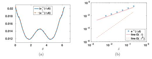
FIG. 6. Panel (a) shows the plot of the absolute value of the far field for both models for  $\delta = 0.05$ . Panel (b) shows the far field  $L^2$  relative error  $e^{\infty}(\delta, d)$ , for different values of  $\delta$ . The approximated rate of convergence is  $O(\delta^1)$ .
