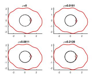
FIG. 7. Reconstruction of a single crack  $\Gamma_0$  in a circular interface, for four levels of noise  $\rho$ . The solid line at the circular interface is the exact location of the crack, and the opening between the dotted lines  $\chi_{\tilde{\Gamma}_+}$  is the predicted location of  $\Gamma_0$ . The outer lighter coloured curve is  $\Gamma_1$ .
