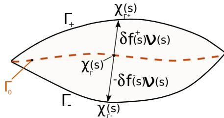
FIG. 2. Zoom of the thin delamination  $\Omega_0$ , and the parametrization of the boundaries  $\Gamma_-$  and  $\Gamma_+$ . Here  $\delta$  scales the width of the delamination and is assumed small compared to other characteristic dimensions of the problem.
