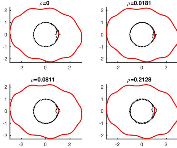
FIG. 7. Reconstruction of a single crack  $\Gamma_0$  in a circular interface, for four levels of noise  $\rho$ . The solid line at the circular interface is the exact location of the crack, and the opening between the dotted lines  $\chi_{\Gamma_0}$  is the predicted location of  $\Gamma_0$ . The outer lighter coloured curve is  $\Gamma_1$ .
