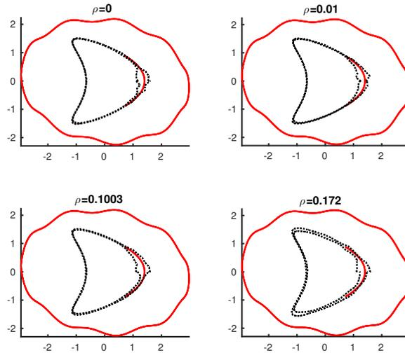
FIG. 8. Reconstruction of a single crack  $\Gamma_0$  in a kite-shaped interface of a two-layered media, for four levels of noise  $\rho$ . The solid line at the kite-shaped interface is the exact location of the crack, and the opening between the dotted lines  $\chi_{\Gamma_0}$  is the predicted location of  $\Gamma_0$ . The outer lighter colored curve is  $\Gamma_1$ .
