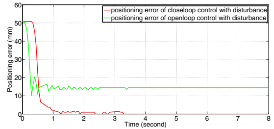
Fig. 4. Comparison of positioning errors between open-loop control and closed-loop control with unknown disturbance
