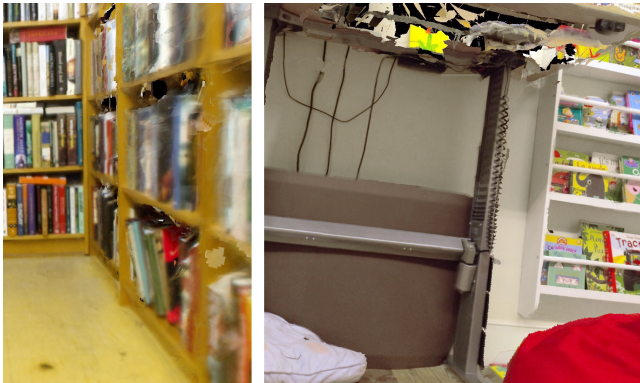
Figure 10: Two typical limitations of our approach: low-resolution texture because cameras that saw these books were far away (left), and missing geometry (right) where the cameras did not look.
