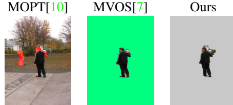
Figure 8: Comparison with a multi-view object segmentation (MVOS [7]). Our approach achieves competitive results without the need for calibration that can be cumbersome in such contexts.
