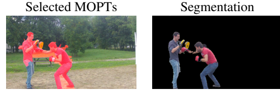
Figure 4: From selected MOPTs to final segmentation. As MOPTs do not precisely delineate moving objects in general, those selected by the proposed method (red overlays) also suffer from such problems. Conducting a final pixel-level segmentation based on selected MOPTs improves the quality of the final results.
