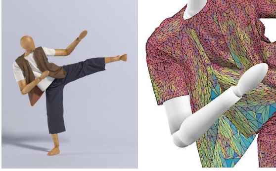
Figure 8: The anisotropic remeshing algorithm of Narain et al. [NSO12] allows detailed wrinkles in cloth to be resolved accurately with fine elements (red), while much coarser elements (blue/green) are used in flat regions. Long, narrow folds are best represented using anisotropic elements (yellow) aligned with the curvature direction.
