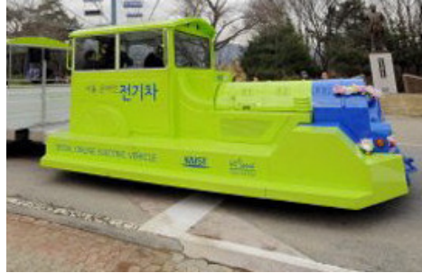
Fig. 4. Street bus with dynamic charging by underground transmitters (KAIST, Korea)
