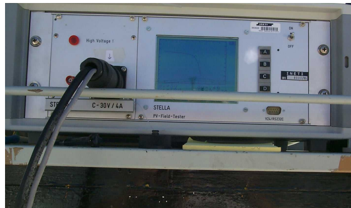
Fig. 3. The I-V curve tracer.
