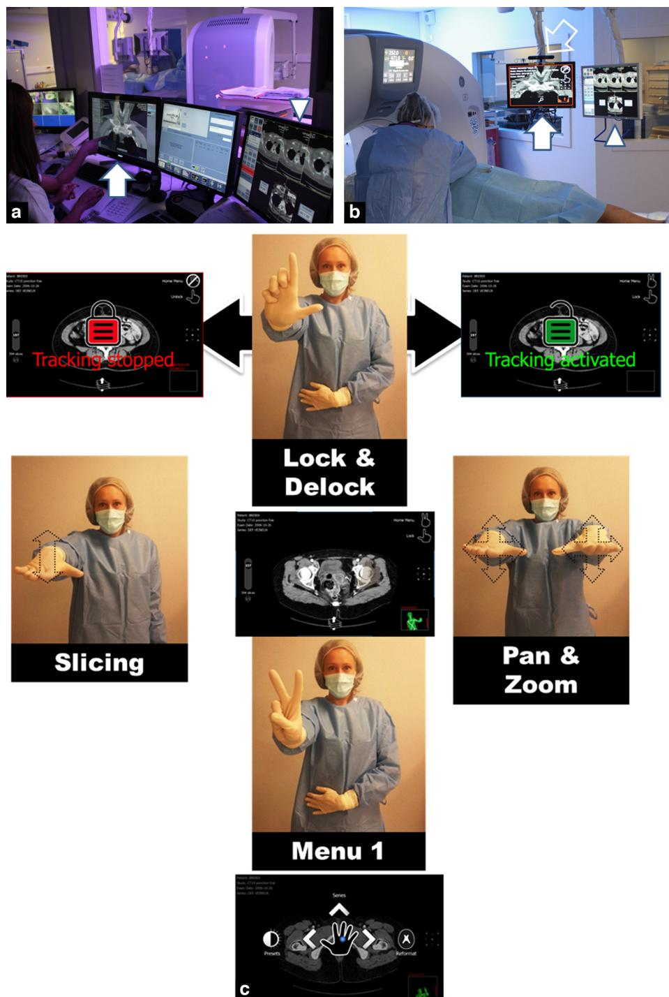
**Figure 1.** Installation of the system in an interventional CT room and operation. a: CT command room with manipulators; b: intervention room, arrowheads = display of images produced during the procedure by the CT duplicated in the intervention room, solid arrows = contactless interface with computer in the command room and full screen duplicated display in the intervention room, hollow arrow = gesture sensor; c: interface gesture semantics.
