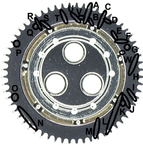
Figure 4. Example of form collecting the labelled anomalies found on a ballbearing. The ballbearing is rejected as defective. The anomalies are evaluated with three intensities (1, 2 and 3), corresponding to levels of increasing seriousness of the anomaly (negligible, possible defect, serious defect).
