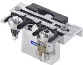
Figure 4: End effector: Parallel Micro Gripper MWPG
