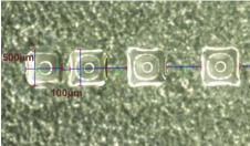
**Fig. 3.** Left: SMD-mask on polymer substrate and plasma nozzle above. Right: Droplets on functionalized surface with  $500\mu m$  edge length and minimal spacing of  $100\mu m$
