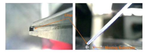
**Fig. 6.** Left: Top view onto the channel with a single chip protruding from the edge. Right: Side view with moving substrate and droplet underneath the chip.
