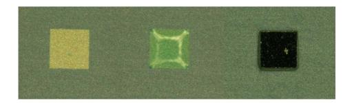
**Fig. 4.** Left: 500µm hydrophile square on an offset-printing plate. Centre: Inked water (for better visualization) on hydrophile area. Right: Self-assembled chip.
