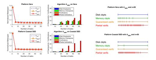
Figure 8: Performance of the three algorithms, and distribution of disk checkpoints, memory checkpoints and verifications (for the  $A_{DMV}$  algorithm) on platforms Hera and Coastal SSD with the *Decrease* pattern.
