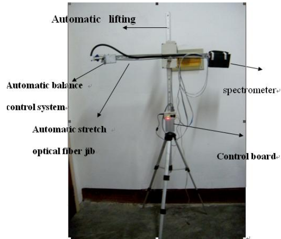
Figure 1. Controllable field spectral measurement device. (China patent of invention 200810180572.7)
