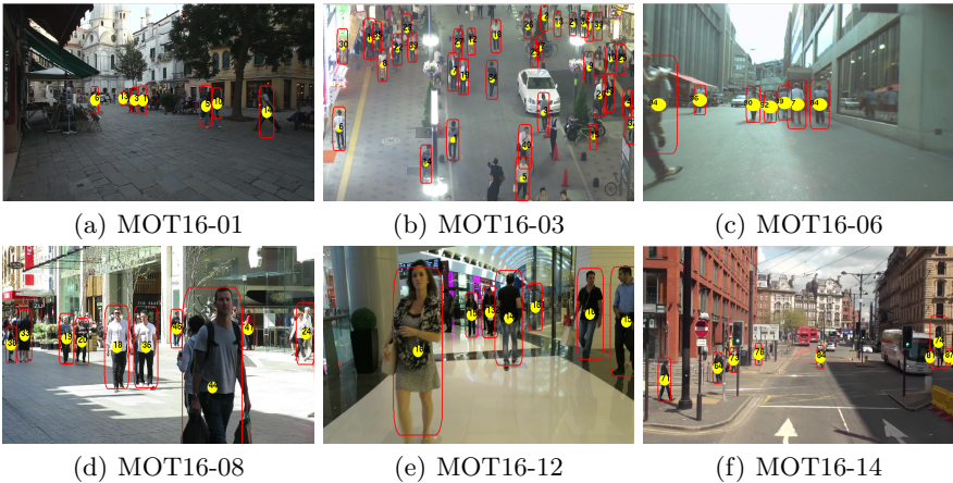
Fig. 3. Sample results on several sequences of MOT16 datasets, red bounding boxes represents the tracking results, and the number inside each box is the track index.
