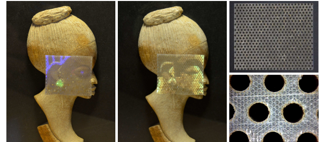
Figure 6: Direct retroreflection: In the left and middle images, we combine the retroreflected augmentation and the view of the object to illustrate our concept of semi-transparent retroreflection. The top right image shows our perforated retroreflective film. The bottom right image shows a close-up where each micro prism is noticeable.
