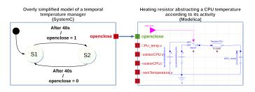
Fig. 4. A simple example mixing SystemC and Modelica
