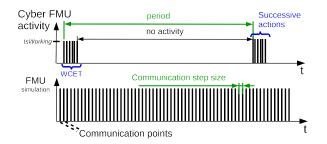
Fig. 8. Problem when using a periodic system with a period >> WCET
