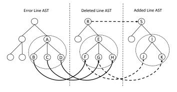
Fig. 4. Code transformation extraction illustration. Error Line AST is extracted from the driver file. Deleted Line and Added Line AST are extracted from historical changes found in the Linux kernel.
