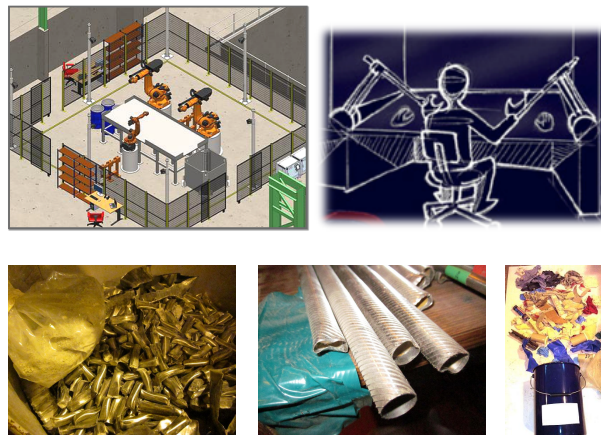
Fig. 1: Top figures: an illustrative sketch of the robotic testbed envisioned for the RoMaNS sort and segregation tasks (left) with a human operator in partial control of the overall motion (right). Bottom figures: examples of the typical waste material to be handled by the robotic cell.
