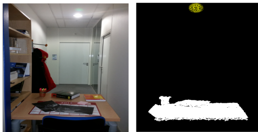
Figure 4: 3D position of the light source. The left image is a captured point cloud of scene and lighting. The right image describes the point cloud of the scene (white pixels) and shows the estimated position of the light source (center of the yellow sphere).
