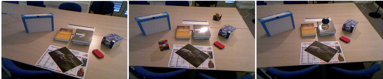
Figure 1: Left: Original captured image of the scene. Center: Augmented scene with two virtual cubes. One can notice the effect of the estimated 3D position of the light source. Right: Augmented scene with a virtual sphere where the specular occlusion is correctly rendered.
