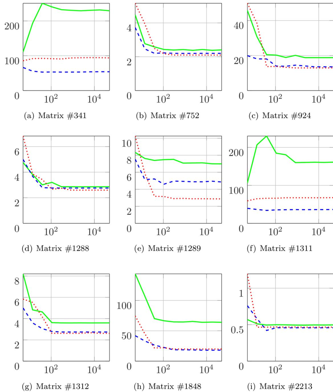
Figure 1: Execution time in seconds ( $y$  axis) of ONLINE-DETECTION (dotted), ABFT-DETECTION (solid line) and ABFT-CORRECTION (dashed) with respect to the normalized MTBF (mean time between failures),  $x$ -axis). The matrix number is in the subcaption.
