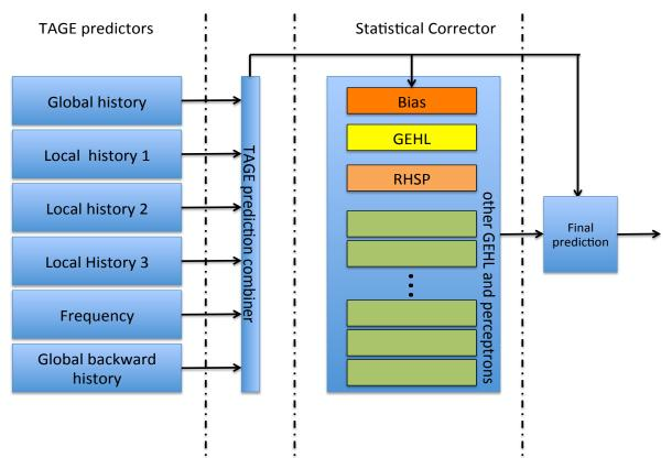
Figure 1: Prediction computation flow on the MTAGE-SC predictor
