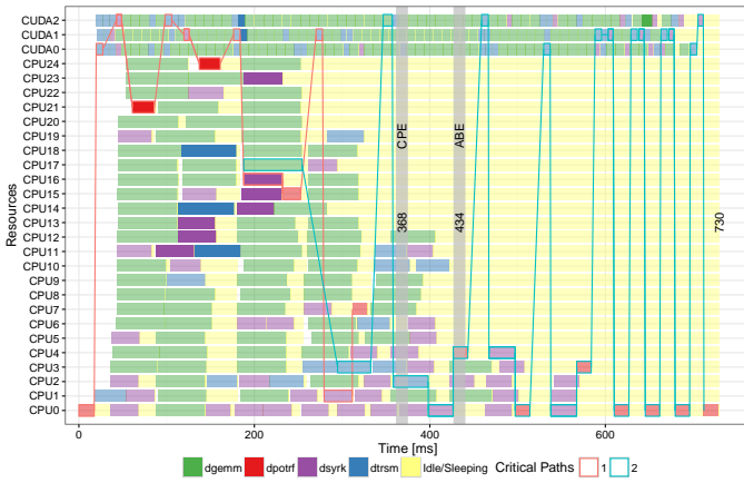
Fig. 5: Detailed view (see http://perf-ev-runtime.gforge.inria.fr/vpa2016/ ) of a 12 \times 12 Cholesky execution (DMDAS scheduler) with two (red and blue) critical paths.
