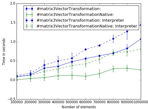
**Figure 2.** Benchmark results for 3x3 matrix vector multiplication.
