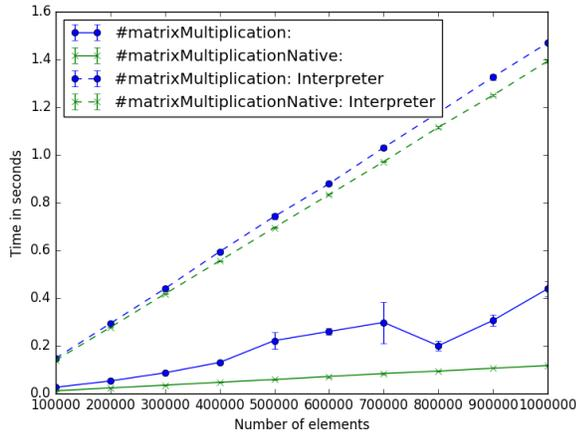
**Figure 1.** Benchmark results for 3x3 matrix-matrix multiplication.
