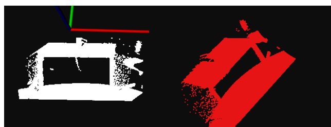
Figure 2: Transformation of a point cloud dataset. The original point cloud, showing a mug placed on a table, is shown in white. The transformed point cloud is shown in red.
