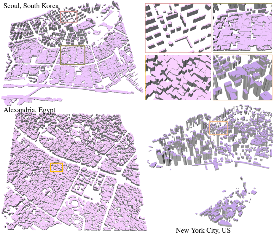
Fig. 10. Reconstruction of cities. Our algorithm performs on different types of urban landscapes, including dense downtown (top left), antique city (bottom left), and US downtown (bottom right). Each model was obtained from one stereo pair of satellite images.
