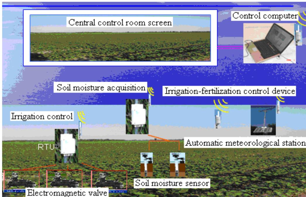
**Fig. 1 Automatic control system in drip irrigation demonstration**
