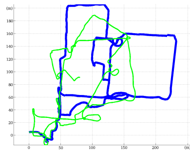
Fig. 18. In green, the trajectory computed using only odometric sensors. The blue trajectory is one given by the GPS and used as a ground truth.
