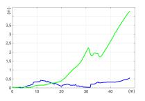
Fig. 10. Root-Mean-Square Error during the trajectory. In green: RMSE of the low-level SLAM. In blue: RMSE with the approach presented in this paper.
