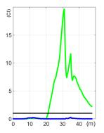
Fig. 11. Consistency Index during the trajectory with associations (zoomed view). In green: RMSE of the low-level SLAM. In blue: RMSE with the approach presented in this paper. The black line represents the consistency threshold.
