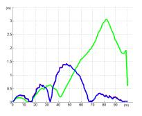
Fig. 4. Root-Mean-Square Error during the trajectory. In green: RMSE of the low-level SLAM. In blue: RMSE with the approach presented in this paper. In red (almost identical to the blue one): RMSE with the previous bias integration.
