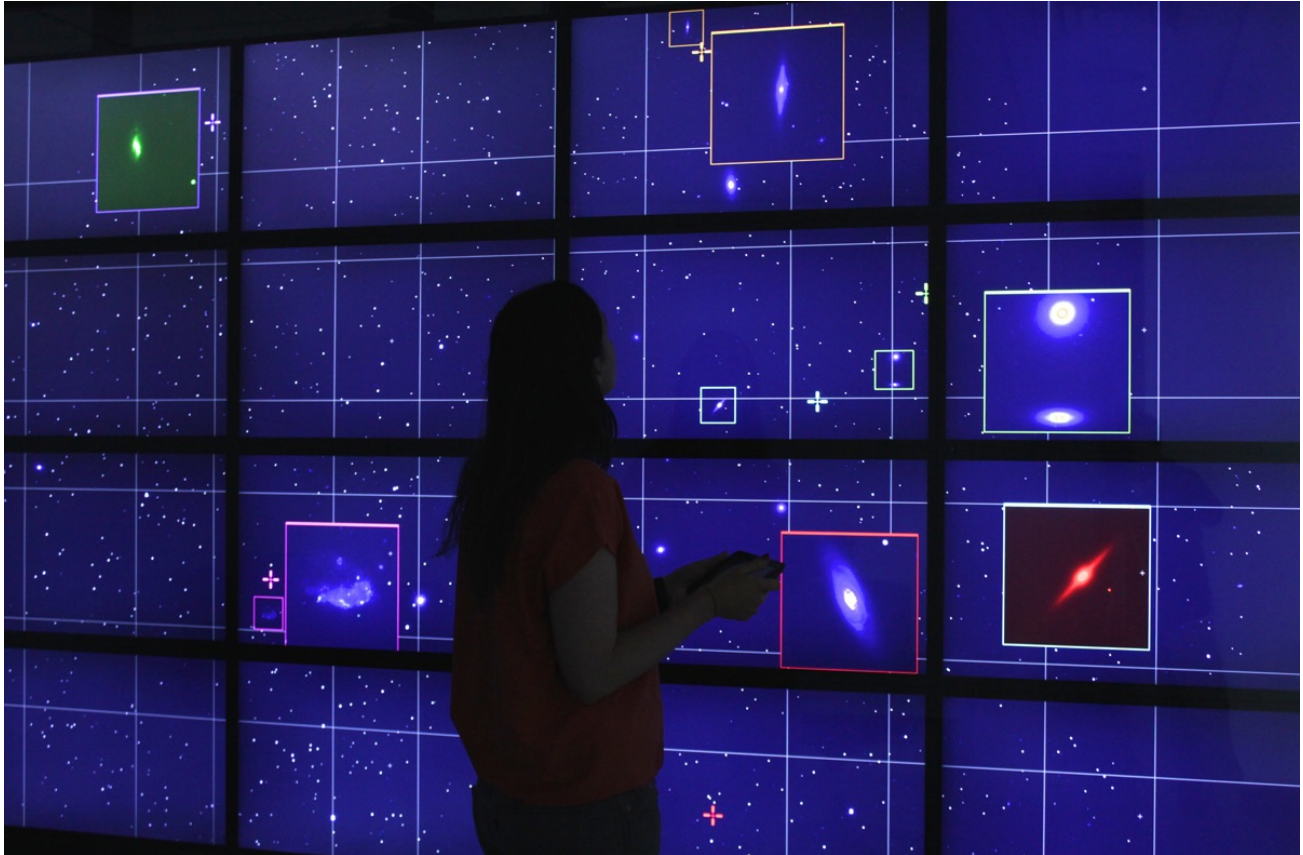
Figure 4. Multiple DragMags magnifying different sources of interest from the same multi-scale FITS image on the ANDES ultra-wall ( 11,520 \times 4,320 pixels) set up at Inria Chile in Santiago.
