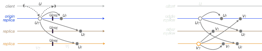
(a) Operation u decomposed into indivisible call, return, generator u_g and effector u_l . Precondition u_{PRE} is true at the effector. (b) The effectors of concurrent operations may execute in different orders in the general case.
