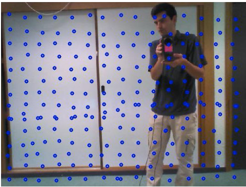
Fig. 3: The audio-visual training dataset contains sound sources emitted by a loud-speaker that correspond to sound directions materialized by image locations (marked as blue circles).
