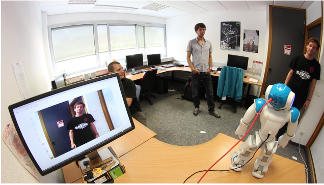
Fig. 2: A typical audio-only localization experiment in the office environment. The robot turns its head towards the speaking person shown on the screen (please see the supplementary video).
