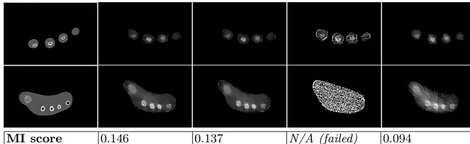
**Fig. 6.** Results on the forearm phantom (2 selected slices and Mutual Information (MI) score). Left-to-right: ground-truth CT scan, proposed method, without optical flow, without  $TVL_1$  prior, ART [8]. Without optical flow, artefacts are visible, for example in the bone cavities. The ART method produces much noisier results.
